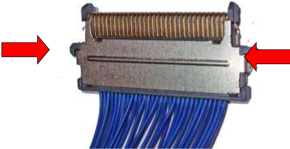
Figure 33: Display Connector Retention Locks
