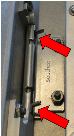
Figure 32: Door Hinge Locked
