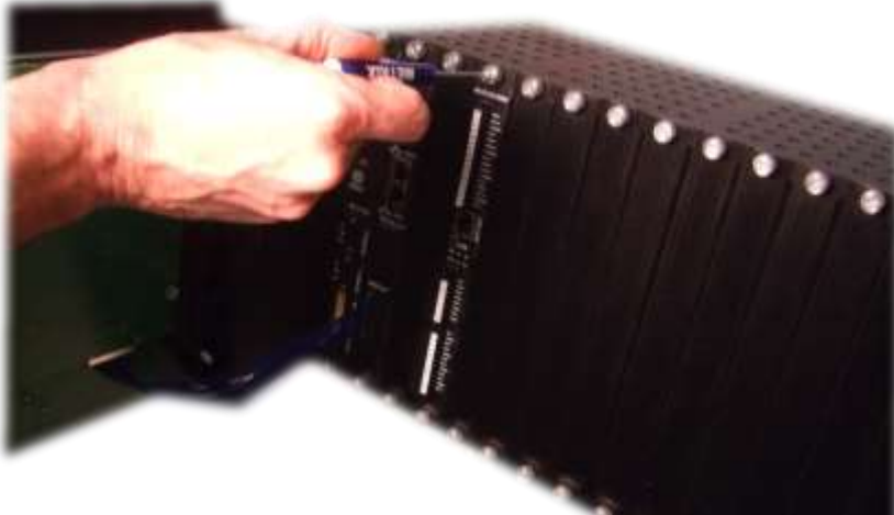
Figure 28: Loosen Captive Screws
